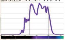
Broad UV spectrum, from 365 nm to 450 nm makes it compatible with all industry standard Etch Resists, Solder Masks and Legends.
