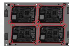
Composite target. To align a single image to multiple sets of hole patterns that have been drilled at different times with potentially different scaling and cordinate origins.
